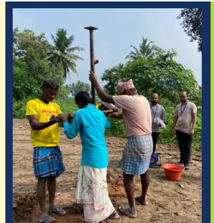
Figure 7: Augur drilling for soil sample collection
